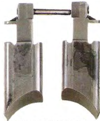
Power Valve Cleanliness Suzuki RM85 Motorcycle Field Test 40 Hours (1 Season Racing Circuit)
